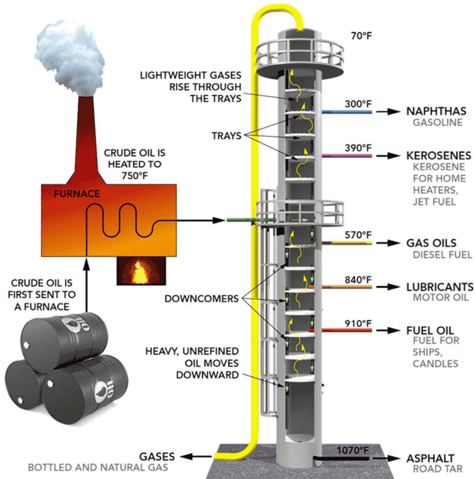
1. Crude oil is heated and introduced into the **Distillation Column**.
