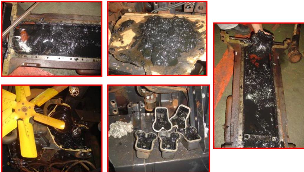
The following pictures will show the damages caused by 200+ hours of use of B-100 biodiesel.
